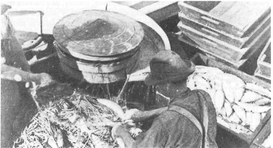
33 A Crossley-type net-lifter, ca. 1925. W.N. Koelz, "Fishing Industry of the Great Lakes," in U.S. Bureau of Fisheries, Report of the United States Commissioner of Fisheries ... 1925 , USGPO, Washington, D.C., 1926, App. 11, Fig. 18.
