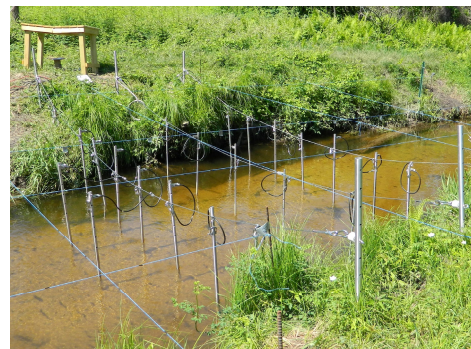
Field test of an electric barrier to block sea lamprey migration.
